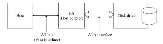
Figure 2.2 1 drive system configuration
